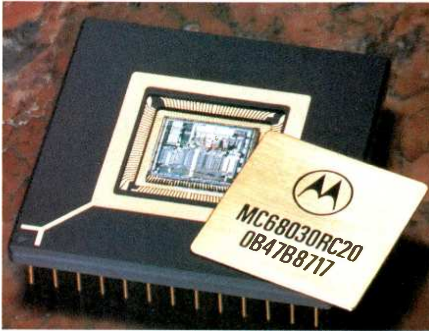
MOTOROLA's 68030 second-generation 32-bit microprocessor.
